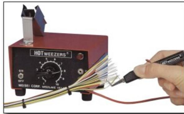
The most unique feature of the HOTWEEZER is that the heater filaments are completely sealed in the stripping head. The head is fabricated from a high-strength, high-temperature alloy with very good oxidation and wear properties. Hermetic sealing of the filaments in a high-temperature alloy offers several advantages:
